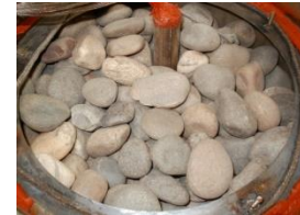
Air-rock bed tests (Denis Okello)
