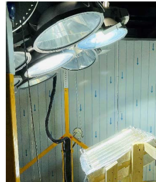
Test with adsorber in refrigeration cycle
