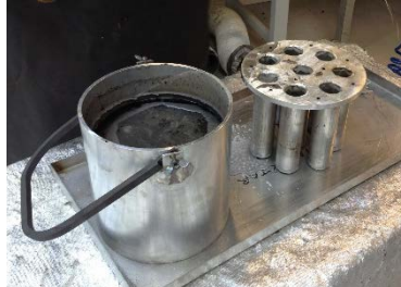
Solar Salt cylinders in heat storage
