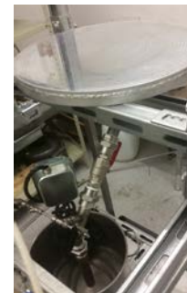
Heat pipe frying pan with evaporator
