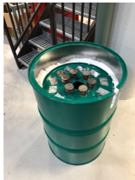
Barrel in barrel with insulation between. PCM cylinders
