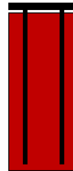
Conducting fins to top cooking plate
