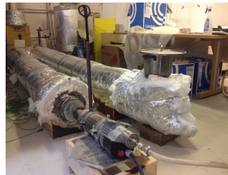
Thermal stratification tests with 8m horizontal and 3 m vertical rock bed
