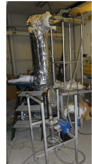
Thermal stratification tests with 8m horizontal and 3 m vertical rock bed
