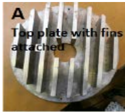
Top plate with hole under cooking pot
