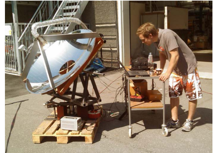
Tests with 300, 600, 900 concentration ratios in dual axis tracking system
