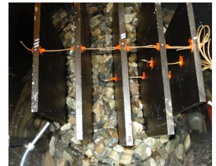
Conducting fins to top cooking plate
